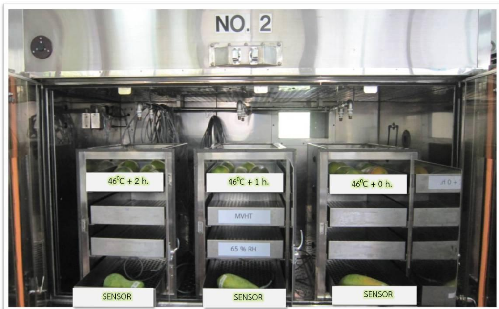
Fig. 3 During treatment : The treatment fruits were placed in the chamber (on top of the metal trays) and monitoring of fruit temperature by using the sensors were placed in the bottom. Two methods VHT and MVHT 65%RH were compared each time by treated fruits until fruit center temperature reached 46 C and held for 0, 1 and 2 h.
