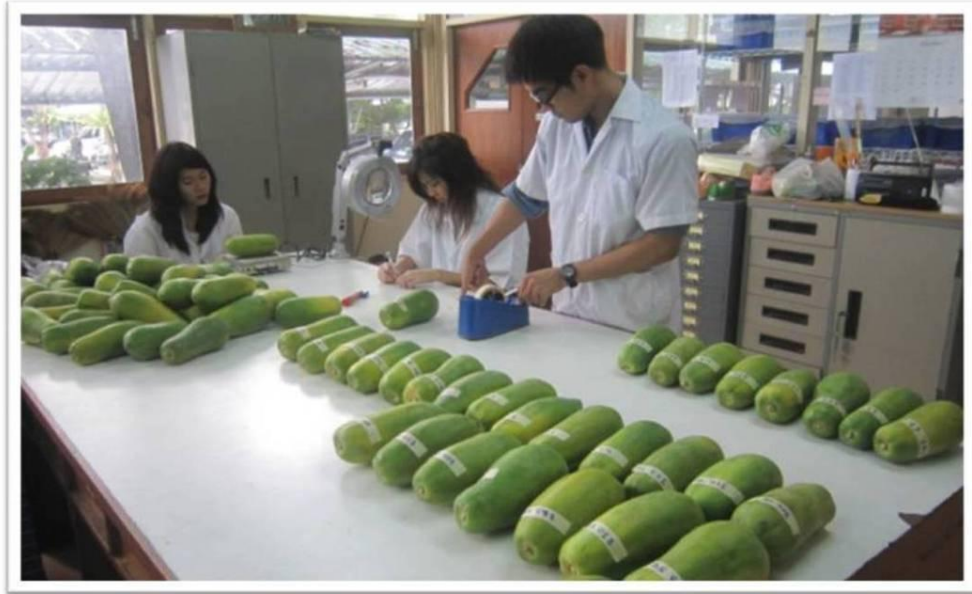
Fig. 2 Laboratory of phytotoxic response of papaya to heat treatment. Before treatment : papayas were weighed, recorded, separated size, label by pen marker and take pictures of fruits.
