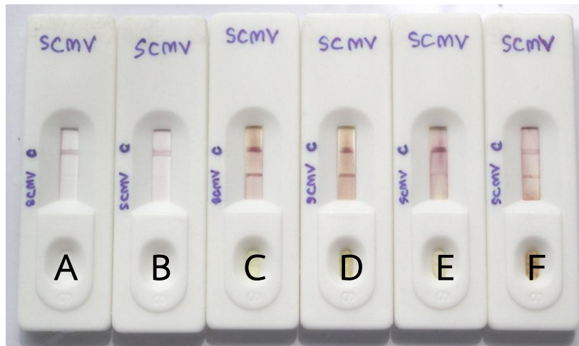
Figure 4 The result of SCMV detection on corn leaves by GLIFT Kit A, B : Negative reaction; purple color stripe in only control line C-F : Positive reaction; purple color stripe in both test line and control line
