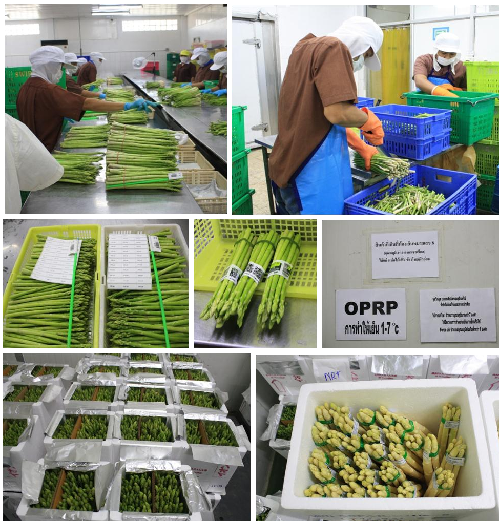
Figure 3 Asparagus packaging method for exportation
