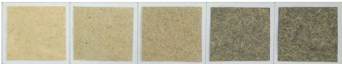
Figure 5 Ethylene absorber paper with various powder AC content; 0, 5, 15, 25 and 35% w/w from left to right.
